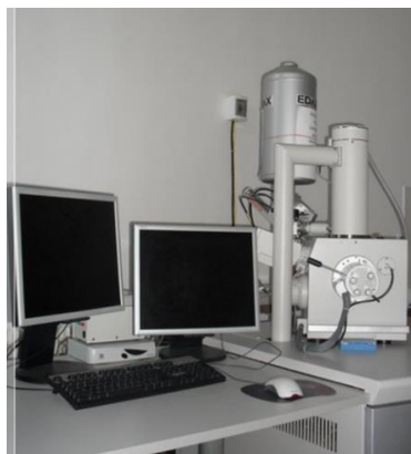
Figura 2.31 Microscopul electronic Quanta Fei 200
