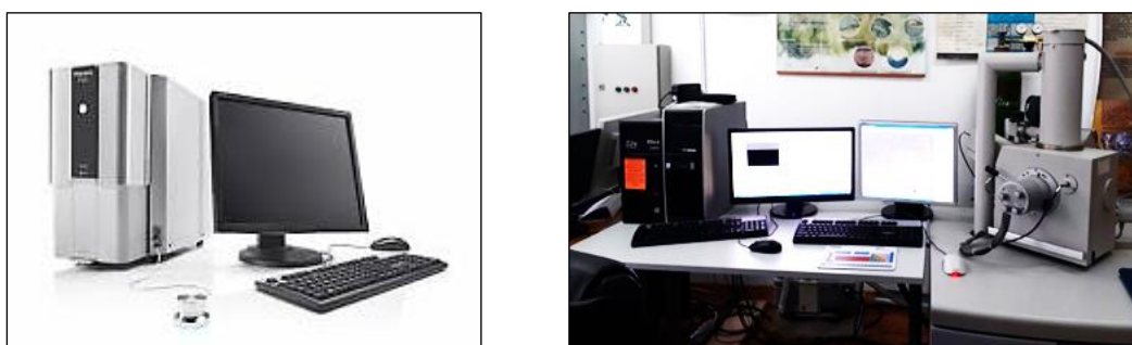
Fig. 2.8. Scanning electron microscope (LAMET Laboratory, UNSTP Bucharest)
